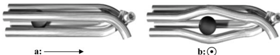
Figure 2 A spherical molecule moving within the polymer matrix and approaching an entanglement: (a) free movement along the axis of a tube; (b) perpendicular movement, requiring sufficient separation of the polymer chains to permit passage of the penetrant molecule to an adjoining tube.
